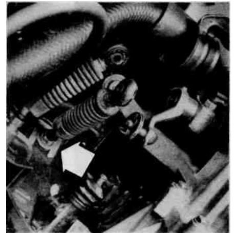
3.5 Both the select and shift control cables are attached to the control cable bracket by small clips identical to the clips used to secure the cables to the shift lever retainer plate — in this photo, the shift control cable clip (arrow) is visible (the select control cable clip is obscured by the clutch bleeder fitting)
