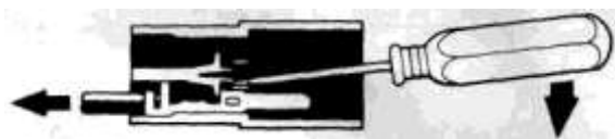
7.16 Pry up the locking lugs with the screwdriver and pull the terminal out from the rear
