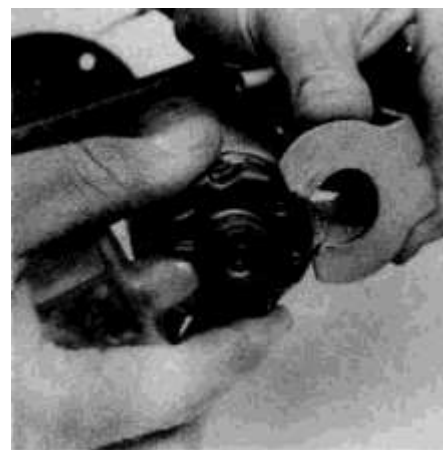
7.7 Pull the lower end of the fuel pump loose from the bracket and remove the rubber cushion that insulates the bottom of the pump
