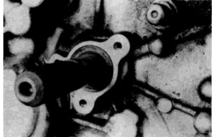
6.4 The input shaft seal is easy to remove with a small screwdriver, but be careful not to scratch the input shaft or the seal bore — when installing the new seal, make sure that seal lip is not damaged by the splined end of the shaft
