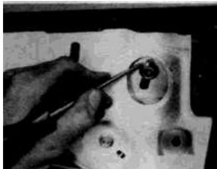
10.3 The guide bolts are located on either end of the door. Mark them for proper alignment during installation, then remove them
