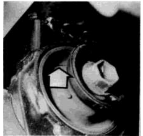
16.3 This hairline crack (arrow) is a typical symptom of an aging mounting insulator that will soon have to be replaced
