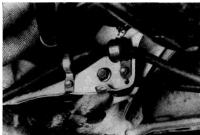
9.4 Remove the strut rod holding nut and bolt along with the cushion
