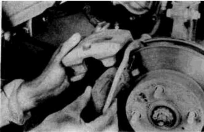
2.4h On the rear calipers, after removing the lower installation bolt, pivot the caliper up on the upper guide pin and separate the pads from the rotor. Note the position of the wear indicator and the other pad components to aid in installation
