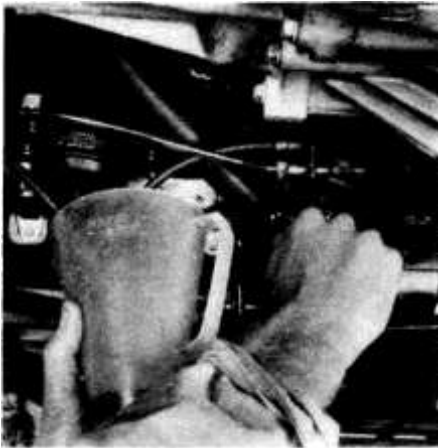
5.3 To bleed the clutch hydraulic system, attach a plastic tube to the bleeder fitting located just to the left of the front transaxle mounting insulator bracket and submerge the other end of the tube in a container partially filled with hydraulic fluid
