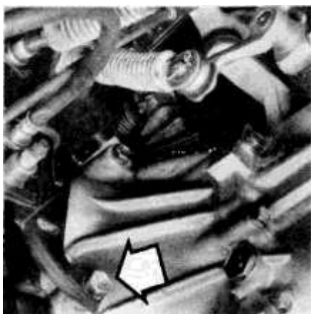
5.13a At its lower end, the control cable bracket is attached to a transaxle-to-engine block bolt (arrow) — remove it . . .
