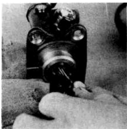
5.10 Push the pistons in and use snap ring pliers to remove the snap ring
