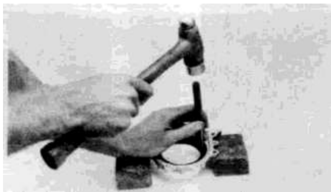
15.6 To remove the old rear oil seal from the retainer, place it on a pair of wood blocks and knock it out with a drift punch and a hammer
