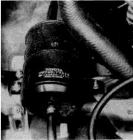
6.3 The charcoal canister is located in the lower left portion of the forward engine compartment firewall
