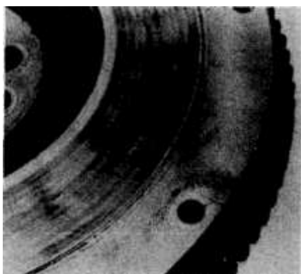
8.6 Carefully examine the friction surface of the flywheel for signs of uneven or excessive wear — if the surface looks excessively worn, it must be either resurfaced or the flywheel must be replaced
