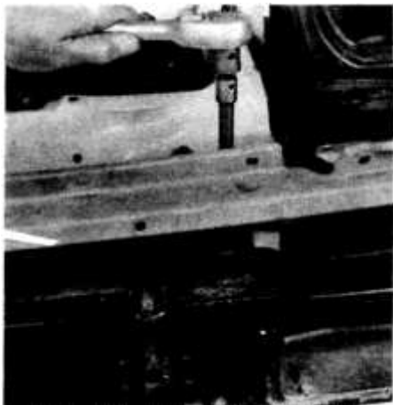
14.7a Remove the two upper bumper bar retaining bolts, one on each end . . .
