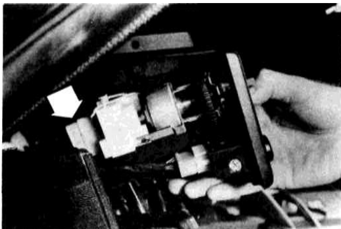
10.3 To check the headlight control switch and rheostat, you must first separate the instrument cluster finish panel from the dash panel, unplug the electrical connector (arrow) . . .
