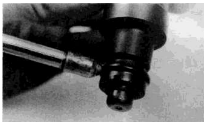
10.18 A little lubrication on the injector nozzle seals makes it a lot easier to insert the injector nozzles back into their bores in the cylinder head
