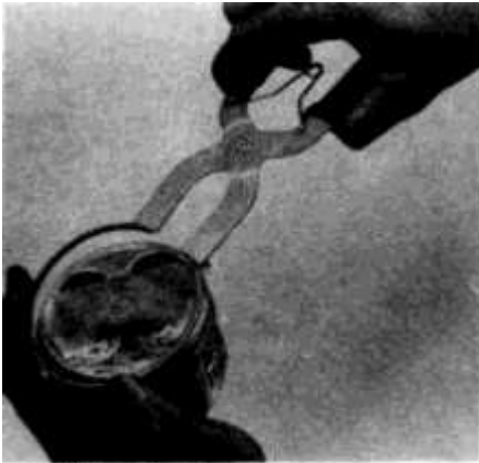
21.10 When installing the compression rings with a ring expander, make sure that the identification mark on the ring faces up
