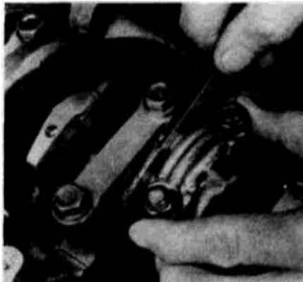
12.3b If a dial gauge is not handy, slip a feeler gauge or gauges, of a thickness equal to the specified end play, between the rod cap and the crankshaft
