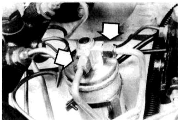
16.2 To remove the accumulator, disconnect the liquid line fittings (arrows)
