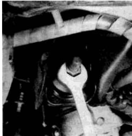
4.3 Remove the strut nut to release the front retainer and cushion
