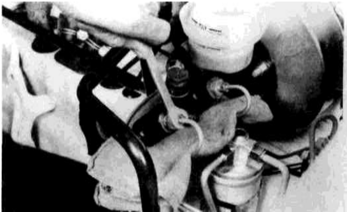
5.4 To prevent rounding the flats on the fittings, use a flare nut wrench to loosen the nuts
