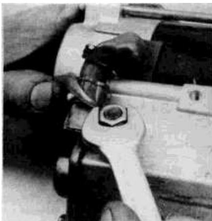
18.3 Remove the terminal nut and disconnect the starter motor lead from the solenoid terminal
