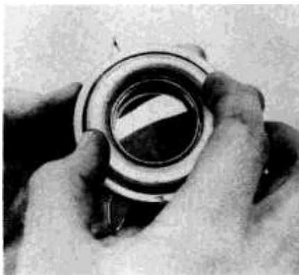
7.8 To check the operation of the throwout bearing, hold it by the outer cage and rotate the inner race while applying axial thrust to it — the bearing should turn smoothly and easily — if it doesn't, replace it
