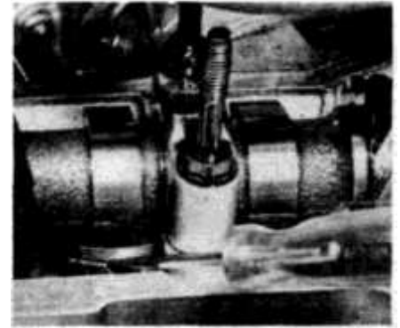
26.9b Remove the shim with a small screwdriver, a pair of tweezers or a magnet
