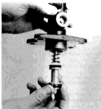
5.11a Tilt the cylinder and remove the No. 1 piston and spring
