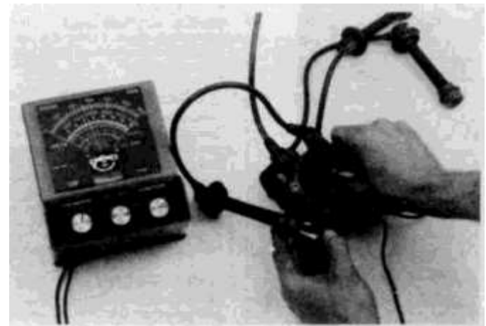
19.13 Measure the resistance value of the distributor cap and the spark plug wires — if it exceeds the specified maximum value, replace either the cap, or the wires, or both
