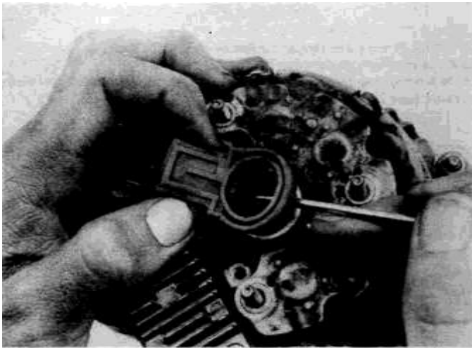
14.7 To facilitate installation of the brush holder, depress each brush with a small screwdriver to clear the shaft
