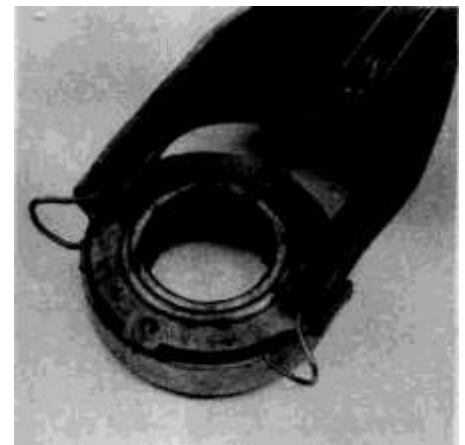
7.4 This is how the throwout bearing spring clip attaches to the backside of the clutch release arm — it's important to visualize this relationship during reassembly
