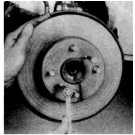
4.6 To help free the rotor, thread the appropriate size bolts into the provided holes. Alternate between the bolts, tightening them several turns at a time until the rotor pops free
