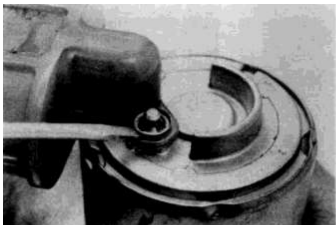
7.9 Pry off the clip holding the strainer to the fuel pump and pull the strainer loose from the pump — replace the clip if it is a loose fit
