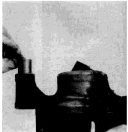
3.8b Push the bushing sleeve out of the caliper
