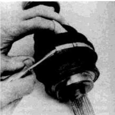
12.3a The large boot clamps can be pried open with a small screwdriver
