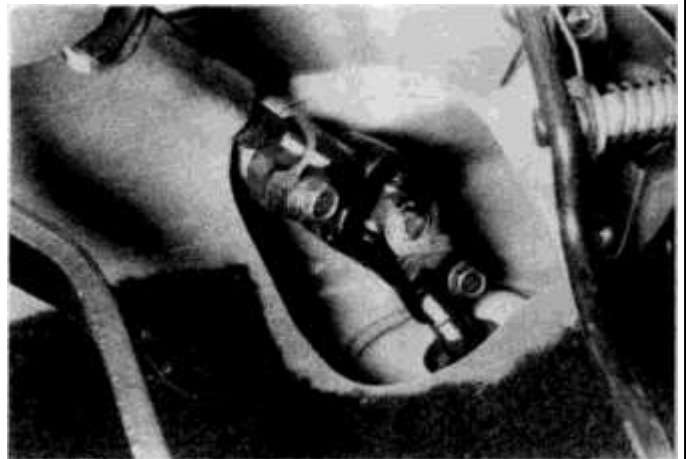
15.4 Paint marks on the steering shaft, joint yoke and pinion shaft to aid reassembly
