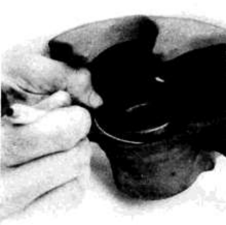
3.4a Using a screwdriver, remove the cylinder boot set ring
