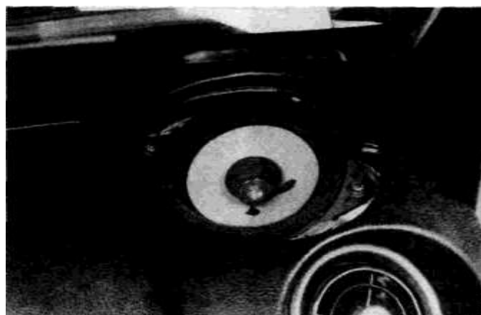
16.7 Remove the two speaker mounting screws, pull the speaker out of the dash, unplug the electrical connector and remove the speaker
