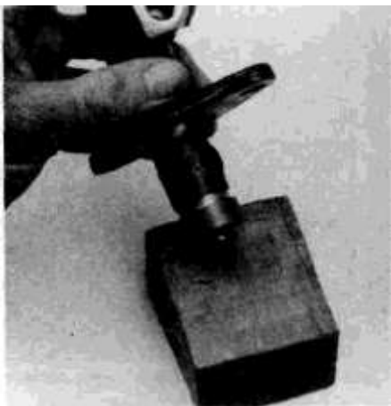
3.8 The piston assembly should come out when the master cylinder body is gently tapped on a piece of wood — if it doesn't, the piston is probably stuck in the bore because of a buildup of varnish or sludge and it will have to be forced out with compressed air
