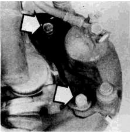
4.5a Remove the two bracket retaining bolts (arrows) to separate the caliper assembly from the rotor
