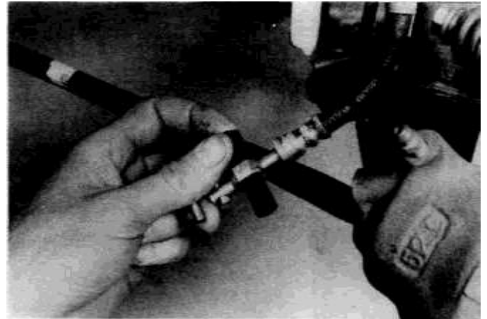
3.1 Using an appropriate sized piece of rubber hose, plug the brake line
