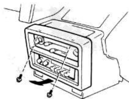
17.13 Take out the two retaining screws and pull out the lower part of the panel
