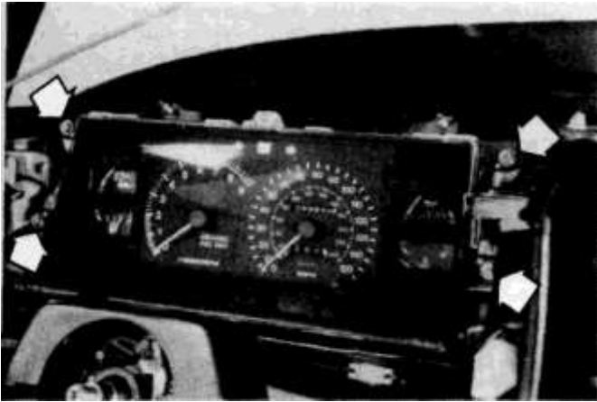
18.2 To disconnect the instrument panel from the instrument panel center reinforcement, remove the four mounting screws (arrows)
