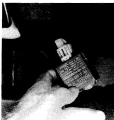
7.1 To remove the turn signal/hazard flasher detach it from the spade connector on top, pull it down and unplug it from the electrical connector
