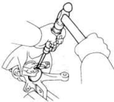
6.13 Clamp the steering knuckle in a vise lined with wood blocks or a soft jaw vise and use a screwdriver and hammer to separate the hub bearing cap and O-ring
