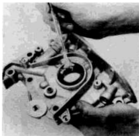
14.6 Coat the lip of the new seal with multipurpose grease so that it won't be damaged by the nose of the crankshaft when the oil pump housing is reinstalled onto the block
