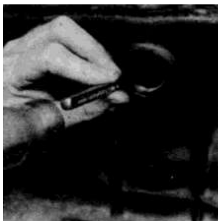
14.1a A hammer and large punch can be used to drive the soft plugs into the block
