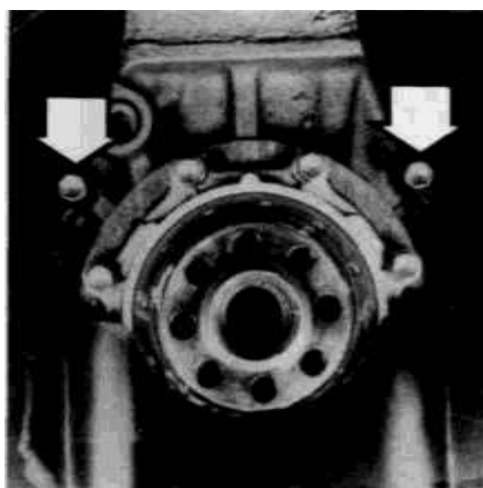
15.3 The rear end plate has to come off before the rear oil seal retainer can be removed — remove both bolts to remove it
