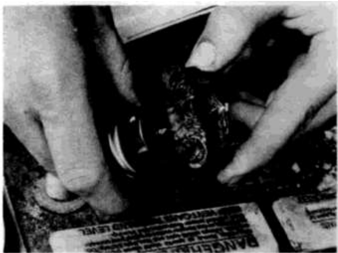
9.7a After washing the cable clamp with a solution of warm water and baking soda, clean it out with a battery brush like this or ream it with a blade type cleaner — remove only enough metal from the inside of the clamp to rid it of any residual corrosion that didn't wash off
