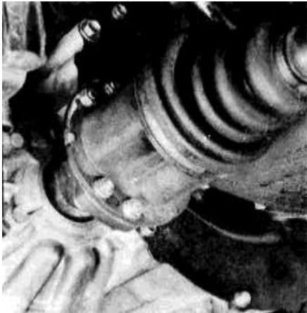
10.8a The inboard joint tulip is attached to the side gear shaft flange with six bolts
