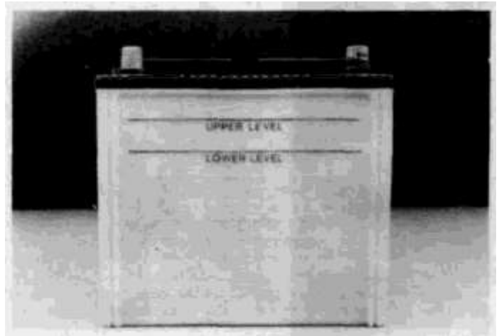
4.15 Keep the electrolyte level of all six cells in the battery between the Lower and Upper levels — use only distilled water to replenish a cell and never overfill it or electrolyte may squirt out of the battery during periods of heavy charging
