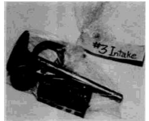
7.2b The preferred method for valve component storage is in a labelled and taped plastic bag
