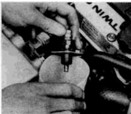
8.5 Place a small container under the cold start injector and turn the ignition key to Start — if the injector is operating properly, it should squirt fuel
