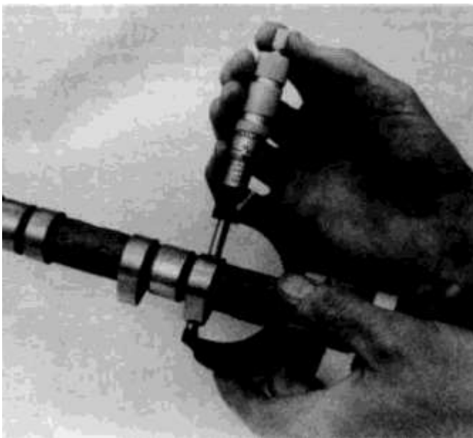
10.1 Measure the lobe height of each lobe on each camshaft — if any lobe height on either cam is less than the specified allowable minimum, replace that cam
