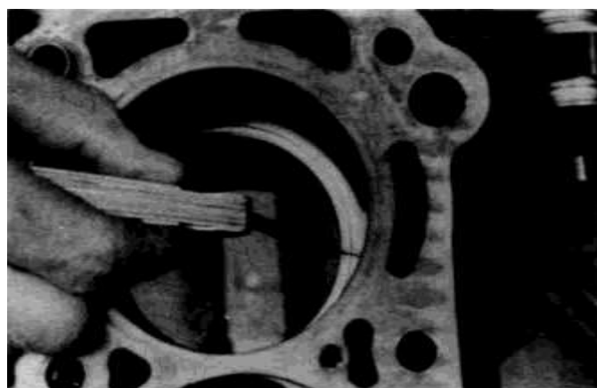
21.4 With the ring square in the cylinder, measure the end gap with a feeler gauge
