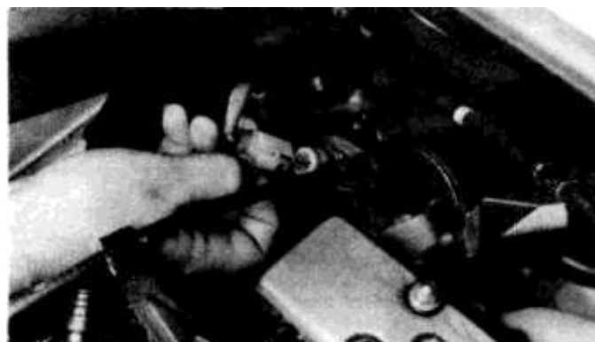
7.2 Locate the temperature sensor and electrical connector on the small bracket at the front left corner of the cylinder head — when this connector is unplugged, the fan should come on — if it doesn't, test the sensor
