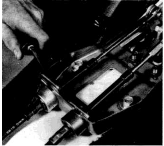
2.4 To remove the shift lever retainer plate, pry both clips loose with a screwdriver — they also have to come off if you intend to replace either or both control cables
