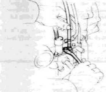
7.16 Push the throttle valve cable into the transaxle case then install the retaining plate and bolt
