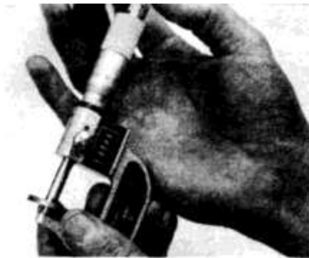
26.10 Measure the shim thickness with a micrometer
