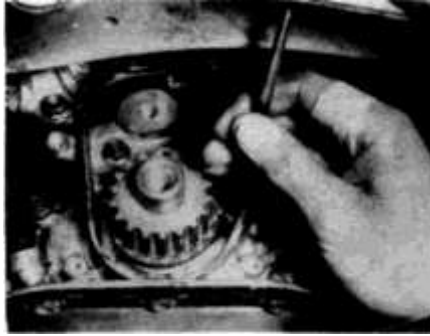
9.31 The crankshaft timing belt pulley can usually be pried loose from the nose of the crank with a small pry bar — if the pulley proves difficult to pry off, take it off with a puller
