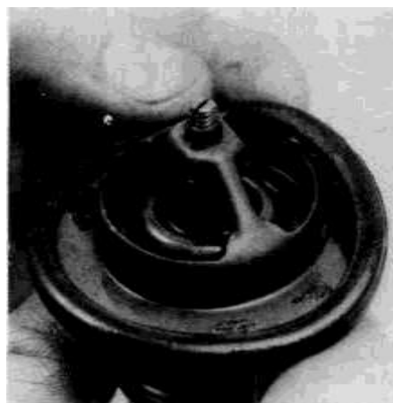
3.6 Be sure to install a new O-ring seal onto the new thermostat
