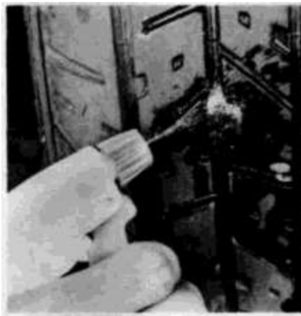
5.4b To look for a leak, spray the suspicious area with a solution of soapy water — if there is a leak in the vicinity, bubbles will appear
