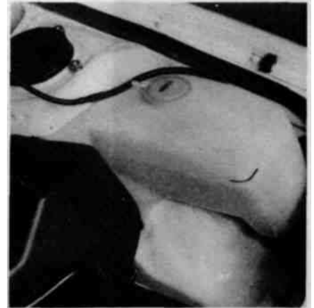
4.14 The windshield washer fluid tank is located in the left front corner of the front compartment — the washer system can use plain water or special washer fluid containing antifreeze to allow operation of the system in climates where the temperature goes below the freezing point
