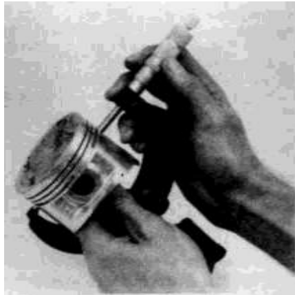
17.11 Measure the piston diameter at a 90° angle to the piston pin and in line with it
